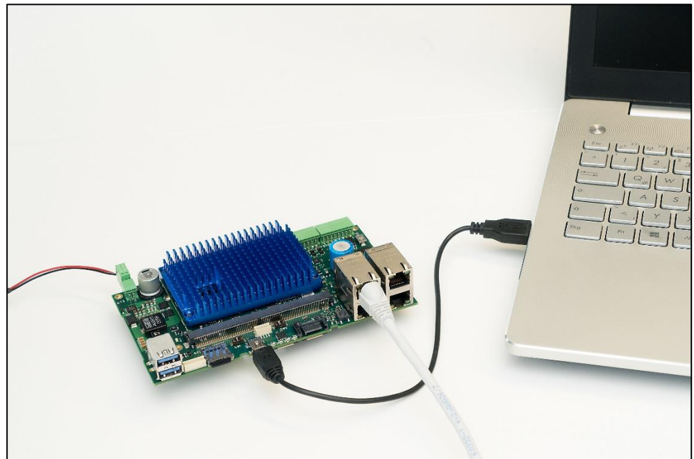
Figure 3-1 System setup example (LAN port 3)
