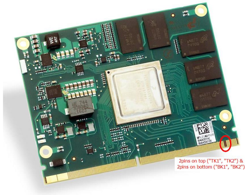
Figure 5-1 Additional Key Pins
