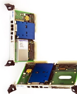
Fig. 2 Optional configurations (with or without mountable drive)
